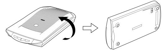
**3** Push the lock switch toward the unlock mark (?).
